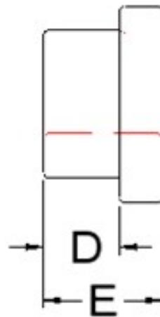
Split Ceramic Eyelets (Flange on one side, split on side for ease of threading)
